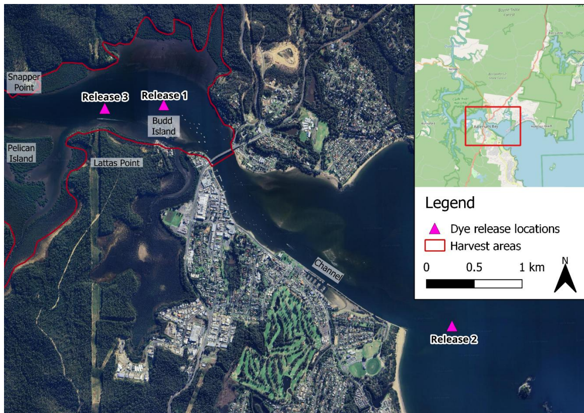
Figure 3-8 Rhodamine WT dye release locations
