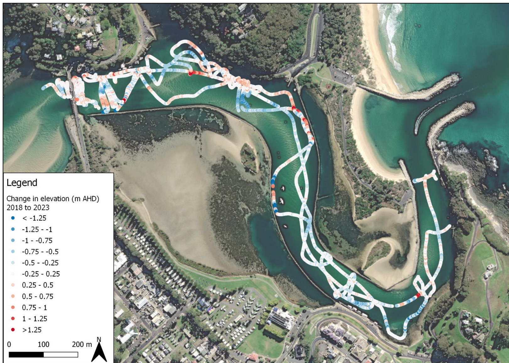
Figure 3-6 Change between 2018 LiDAR and 2023 fieldwork bathymetry. Blue corresponds to erosion and red accretion
