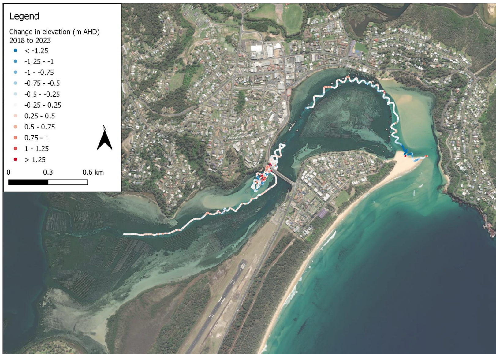
Figure 3-6 Difference between 2018 LiDAR and 2023 fieldwork bathymetry. Red corresponds to accretion and blue to erosion
