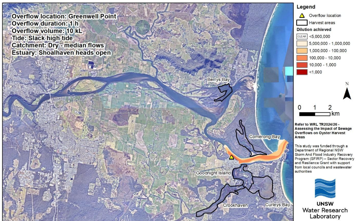
Figure 7-5 Modelled spill from Greenwell Point on a slack high tide with D = 0.5 \text{ m}^2/\text{s}^* *Result figures present the minimum dilution (i.e., maximum concentration) observed at each point during the entire scenario period (21 days).
