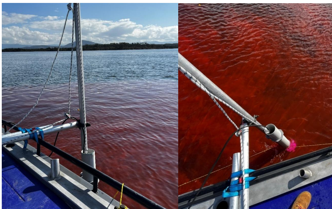
Figure 4-3 Setup with C3 Fluorimeter used for tracing Rhodamine WT
