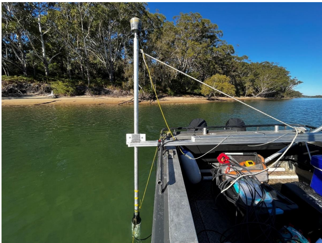
Figure 4-1 Boat mounted Sontek M9 ADCP (in water) and RTK GPS (top)
