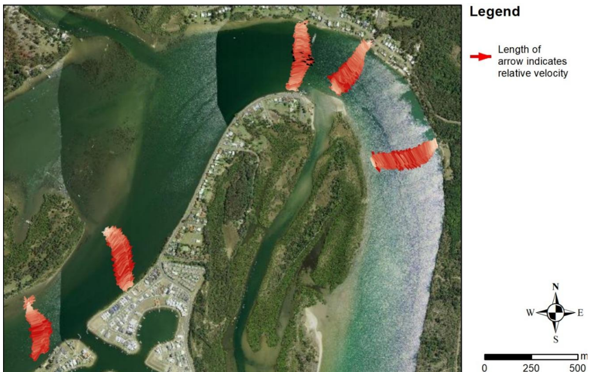
Figure A-6 Velocity distribution on an outgoing ebb tide
