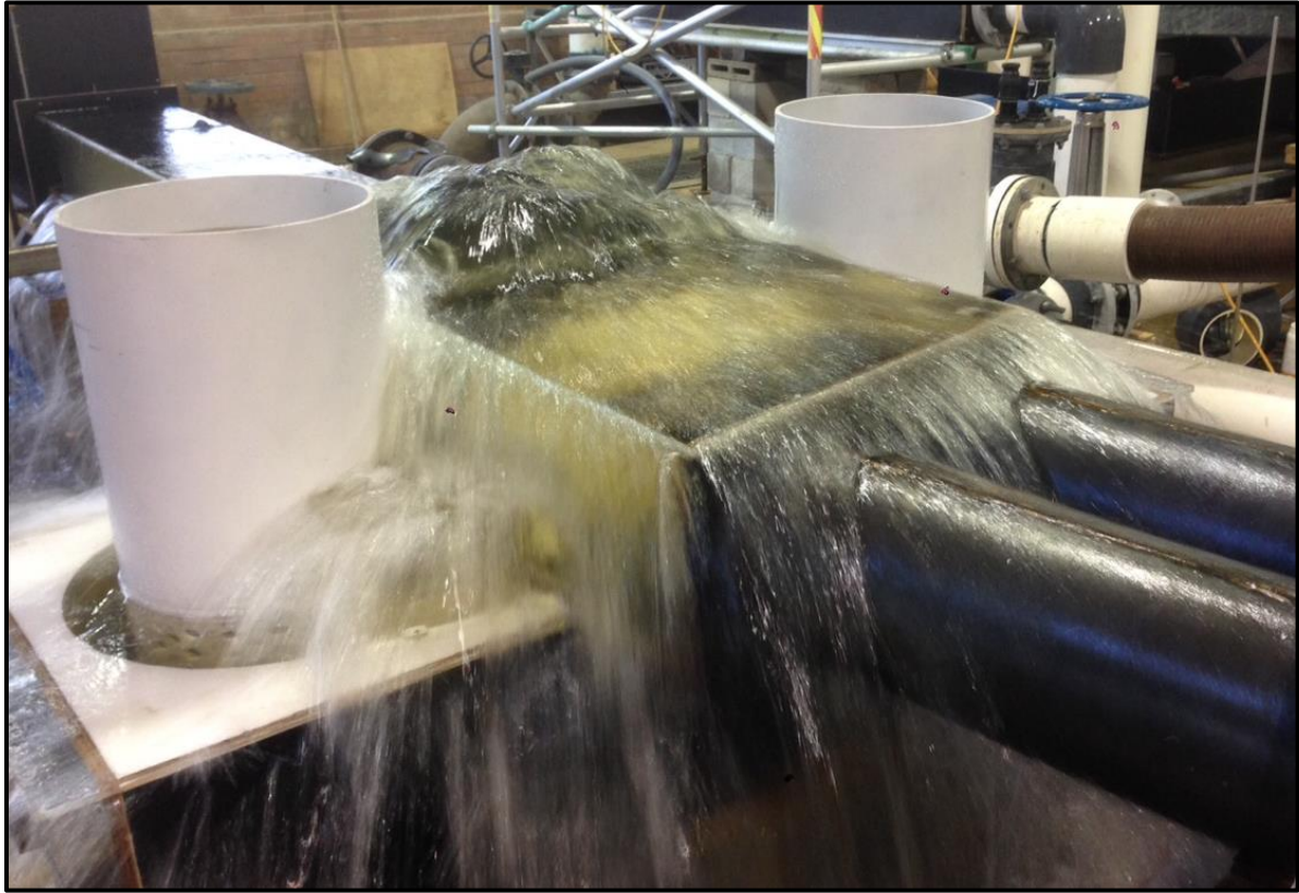
Figure 4 – Water Surcharging During 100 year ARI 2m x 2m Grate Test
