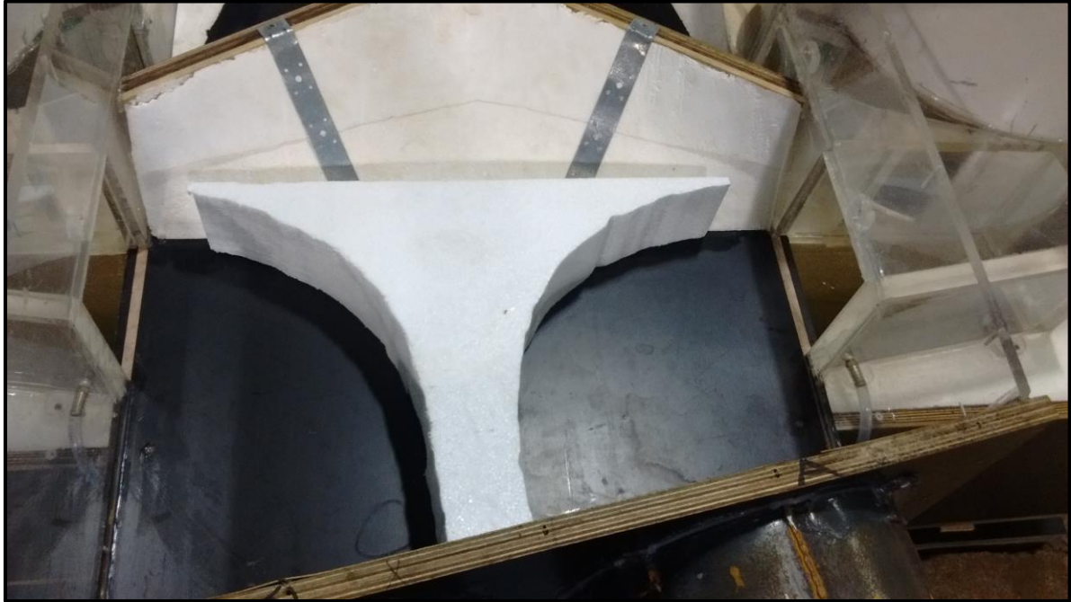
Figure 6 – Benching Trial in Downstream Section
