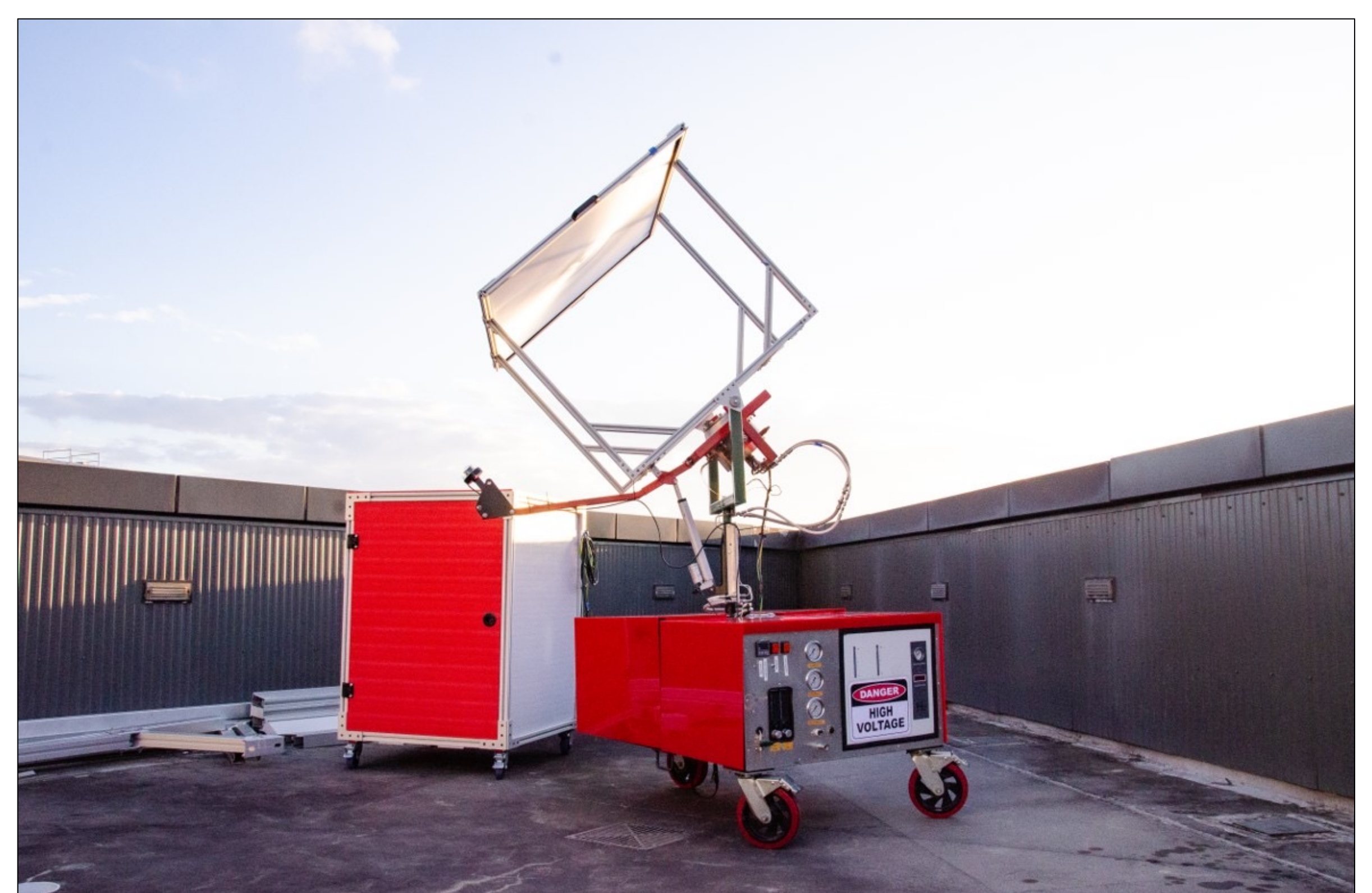
SHINE 2.0 (Solar Harvesting for Integrated New Energy) produces hydrogen using concentrated sunlight to directly heat a methanation reactor beside a solar photovoltaic panel that generates the necessary electricity. The hydrogen is fed with captured carbon dioxide to produce valuable methane.
