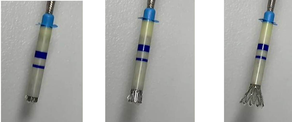
Figure 51. The Release Process of Stent
