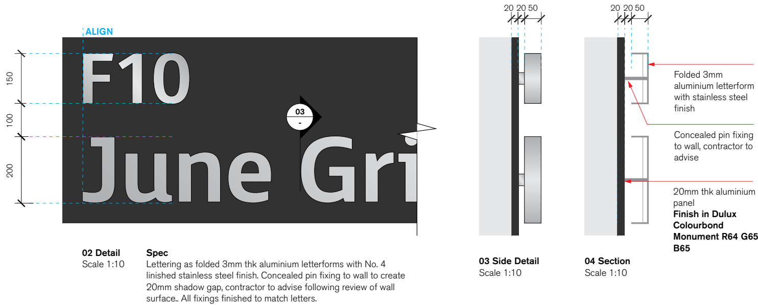
01 Elevation Scale 1:25 Note Elevation drawn indicatively only, contractor to confirm all dimensions onsite and provide accurate setouts in shopdrawing issue. Existing building identification (shown on previous page) is to be removed and concrete wall is to be cleaned and made good prior to installation of new lettering. Any existing regulatory signage is to be relocated, per contractor's onsite review.
