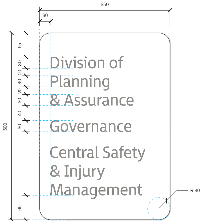
02 Detail Scale 1:5 Spec Panel as 3mm thk acrylic with 2 pac polyurethane finish to match Dulux 'Vivid White' SW1G1, adhesive fixed to nominated door or wall surface. Graphics and messaging to be profile-cut 3M Scotchcal self adhesive vinyl in Mid Gray 61 applied to panel surface.
