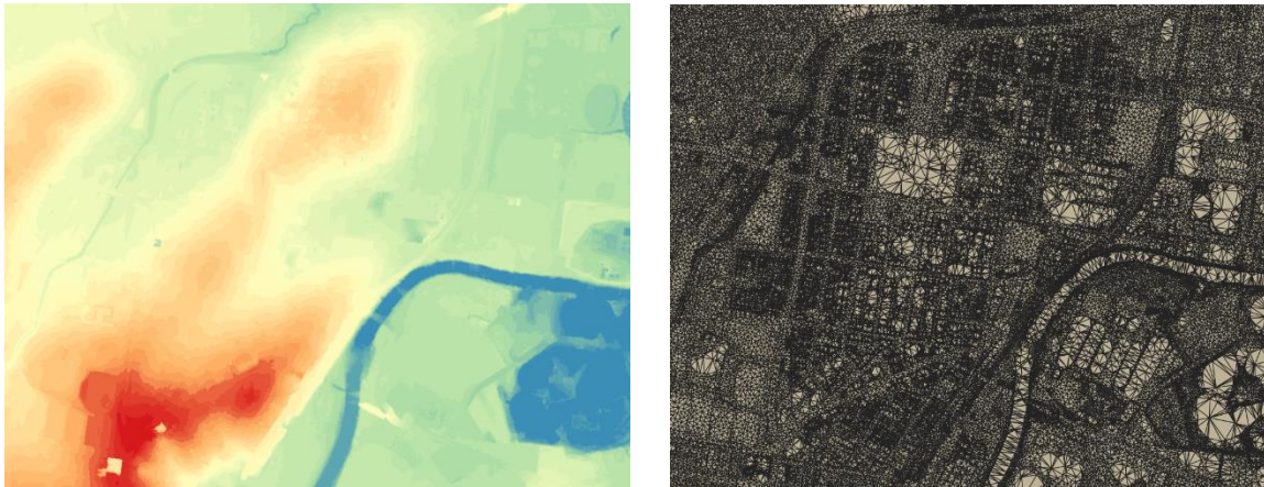
Figure 7: Coloured DEM (left - blue is the lowest elevation and red the highest), derived TIN (right).
