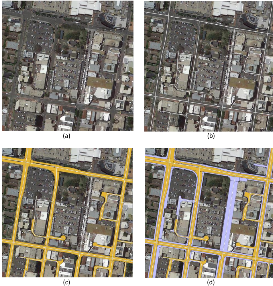
Figure 11: Different Road datasets. (a) Satellite image of a selected area in LCC. (b) 3D road line dataset (white). (c) PMS road dataset (yellow). (d) Road cadastre dataset (purple).
