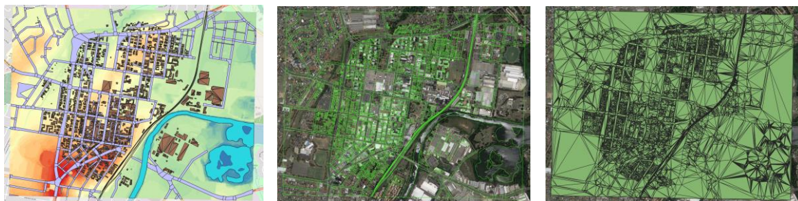
Figure 17: All the features in the selected sample area (left). The extracted 3D boundary lines of the features (middle). Generated TIN (right).
