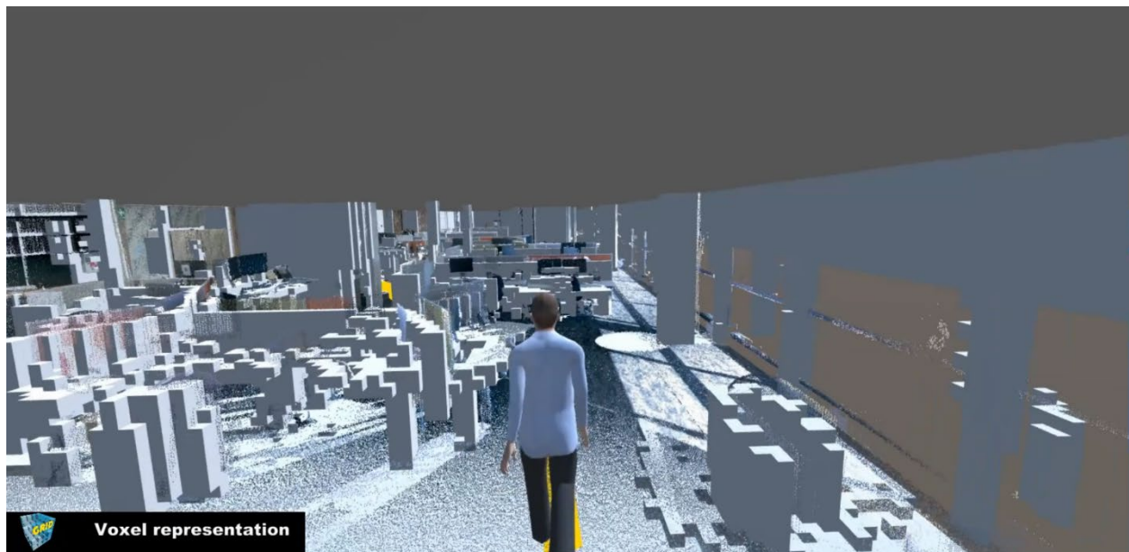
Figure 9: Using voxel-based model for indoor navigation
