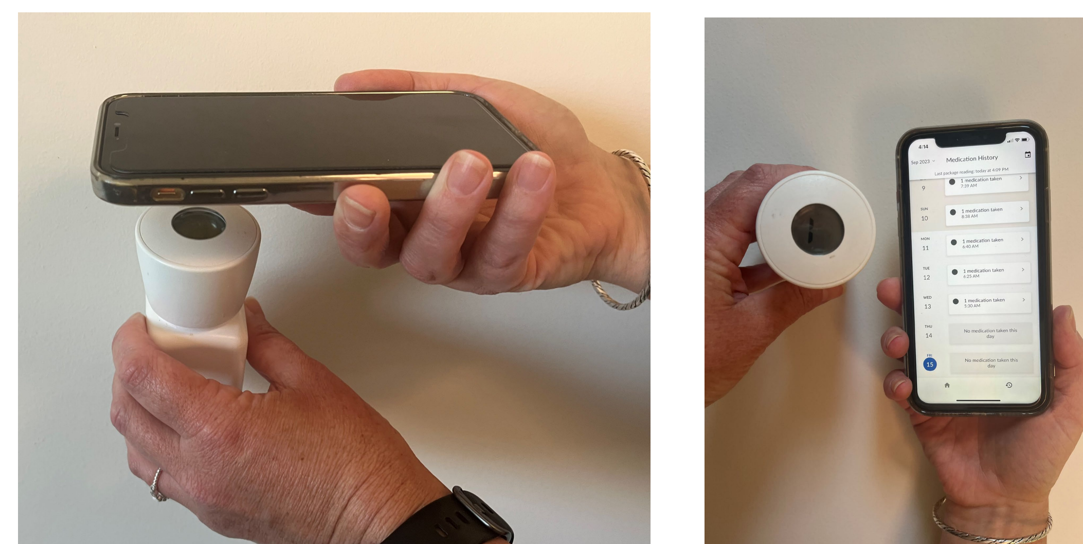
Figure 3. Uploading adherence data from the MEMS Smartcap® using a Smartphone with Near Field Communication
