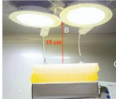
Figure 1: Test set up for testing the C-Guard Non-UV lights
