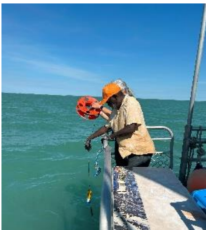
Traditional owner Simon Peter Munkard collecting temperature data using a Moana sensor on a hand reel. Credit: M. Roughan.
