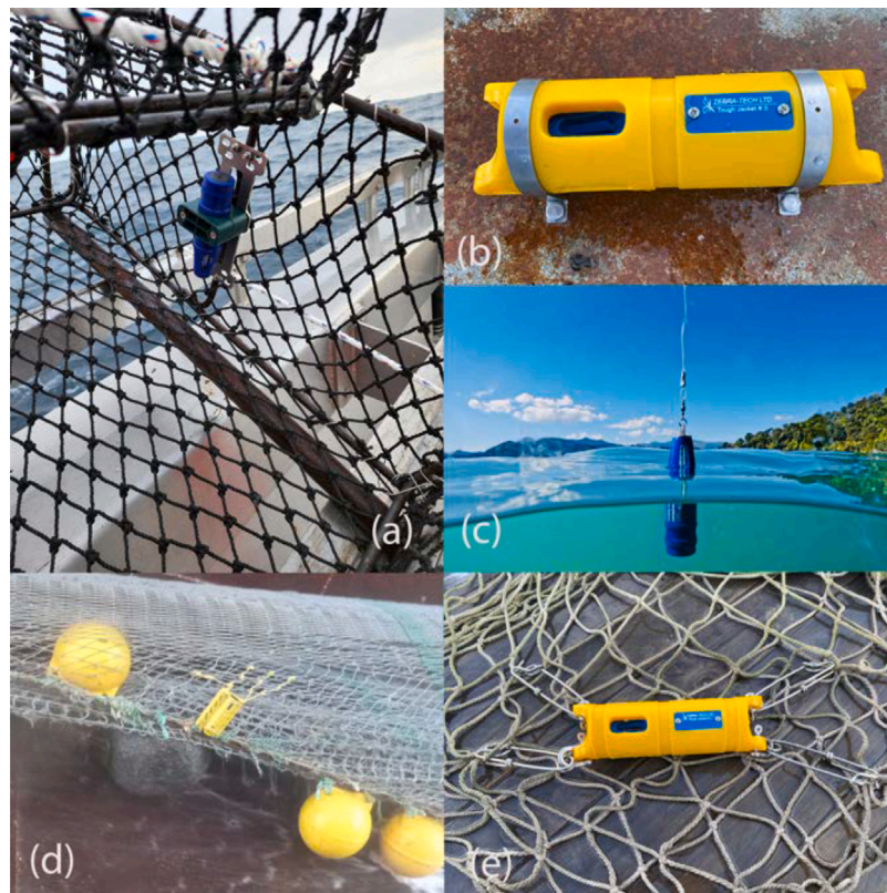
Fig. 4. Sample Mangōpare sensor (blue), or sensor within a protective “tough jacket” (yellow), installation on a (a) lobster pot, (b) trawl door, (c) fishing line, (d) mounting plate on net, and (e) shark clips on net. Additional mounting options, not shown here, are currently in use by the commercial fishing fleet. Photos are courtesy of: (a) William Maclardy, (b) John Radford - ZebraTech, (c) Amanda Rudkin, (d) Talleys Group Ltd., (e) John Radford - ZebraTech.
