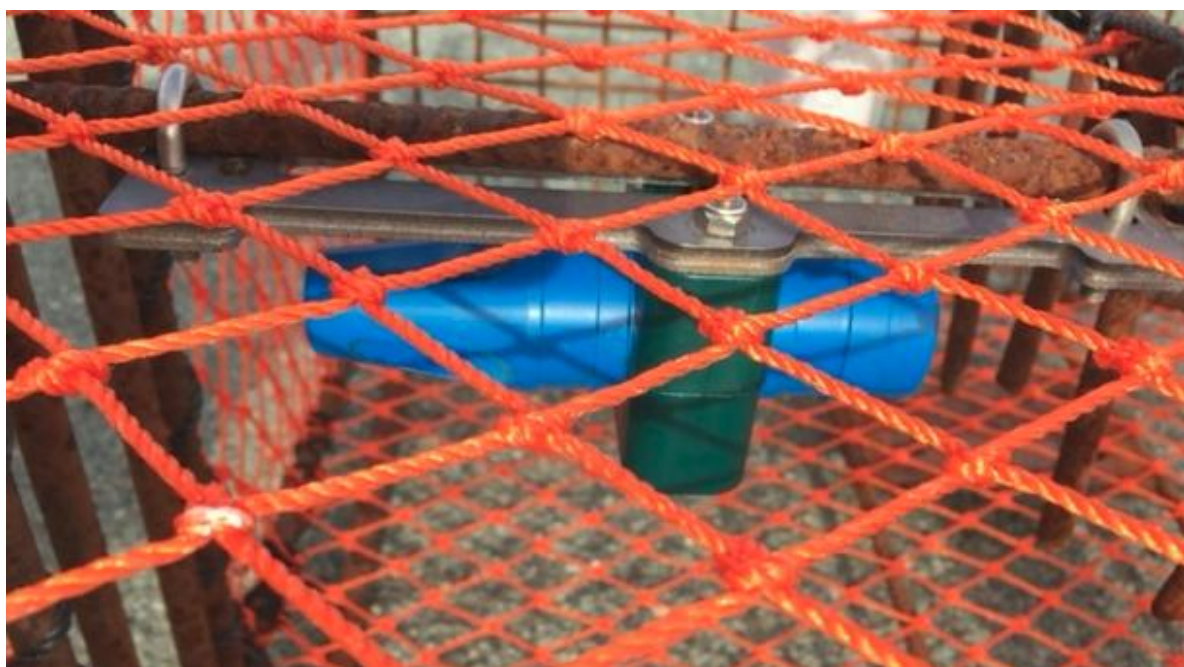
Photo 3. Moana TD mounted inside a fishing pot
