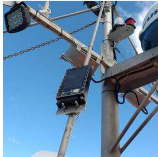
Photo 8 & 9. Deck Unit mounted at 45 Degrees to minimise heating in hot climates
