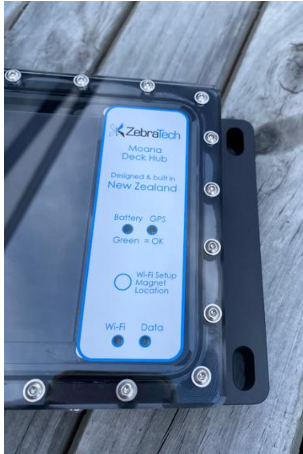
Photo 12. Deck Unit status indicator panel
