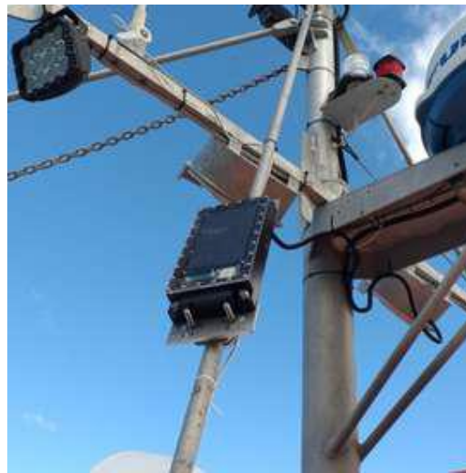
Photo 9 & 10. Deck Unit mounted at 45 Degrees to minimise heating in hot climates
