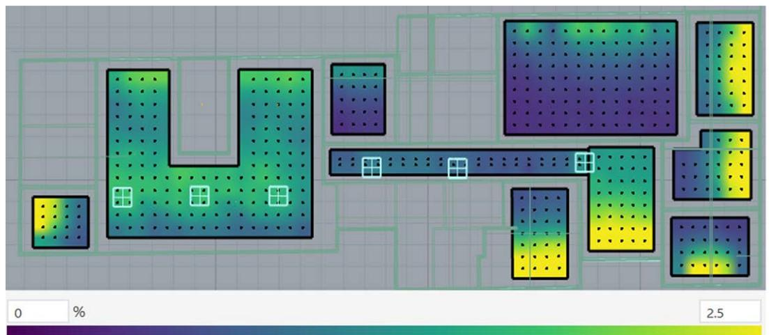
Figure A1. Distribution of Average Daylight Factor in continuously occupied spaces
