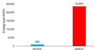
Figure 8. Whole building energy gain for heating and cooling load – heating season (May-September).
