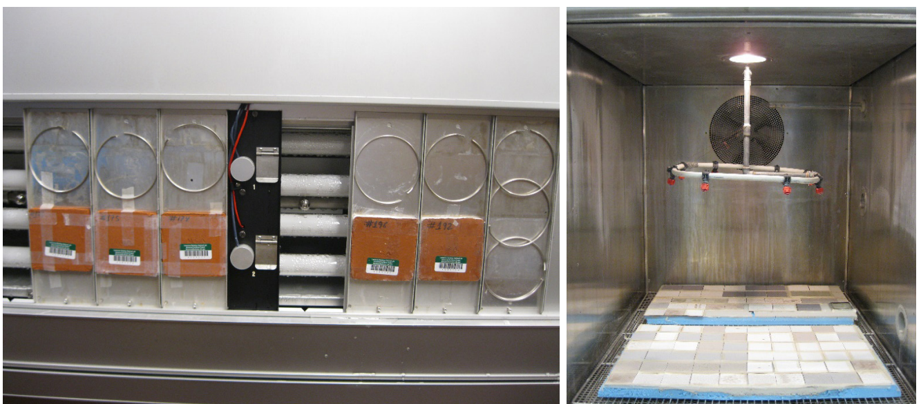
Figure 5.8 Examples of different weathering chambers for laboratory exposure to UV radiation and variations in temperature and humidity, and rain.
