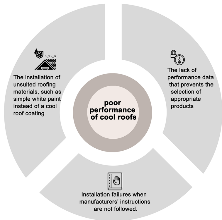
Figure 2.9 Causes of poor performance of cool roofs.
