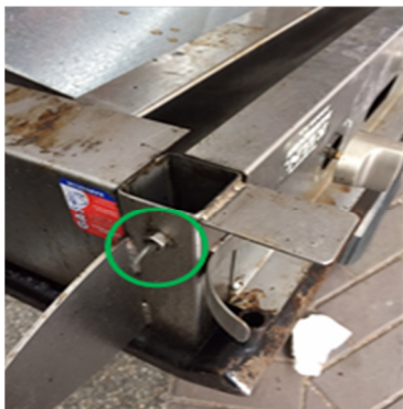
Photo 1: hand tightened flat head screws used to hold on the barbecue legs
