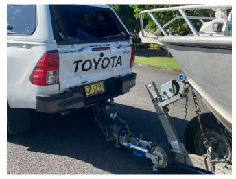
inserting the safety pin into the coupling latch of the trailer
