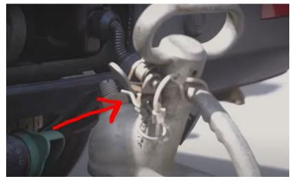
coupling latch to lock in the connection mechanism for the trailer
